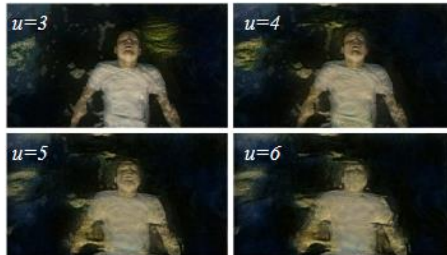
Figure 6: Increasing the value of u gave us a control to fine-tune the degree of subjectively-measured impressionism present in the style transfer
